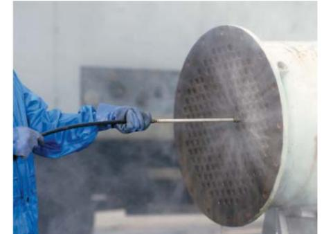
Cleaning of heat exchanger with Spin Nozzle.
